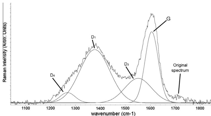
Fig. 6. Raman spectra of kerogen extract isolated from chert sample in which carbon Raman absorption bands can be identified.
