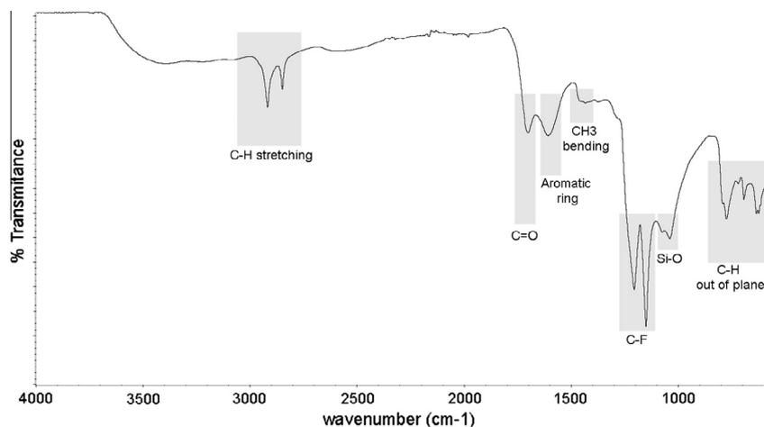
Fig. 5. ATR-IR spectra of isolated kerogen which shows the typical characteristic infrared bands of this compound.
