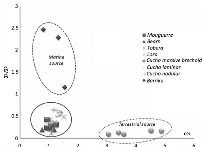
**Fig. 1.** Light/heavy *n*-alkane ratios ( $\sum 1/\sum 2$ ) vs. Carbon Preference Index (CPI) diagram showing the different *n*-alkane profiles found in the analysed chert samples.
