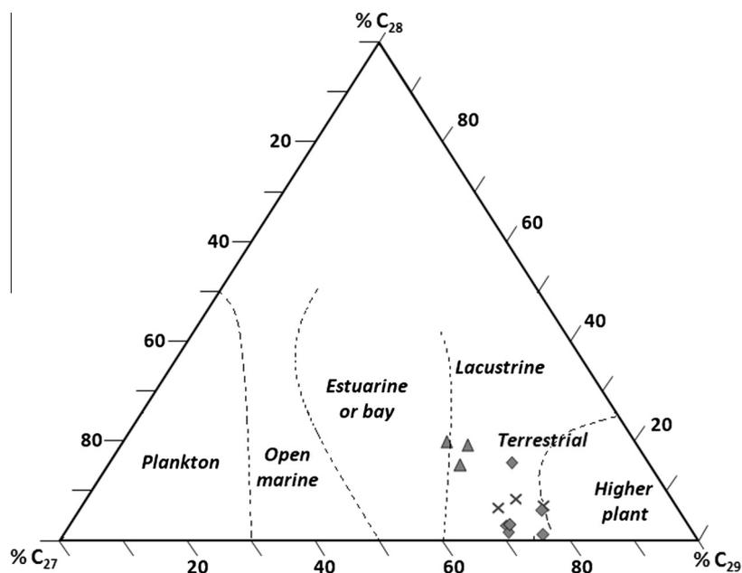
**Fig. 4.** Sterane ternary diagram as a function of sterol compositions in analysed chert samples collected in *Cucho*: laminar ( $\blacktriangle$ ), massive-brechoid ( $\times$ ) and nodular ( $\blacklozenge$ ). The dotted zone underlines the different environments characterised by sedimentology.
