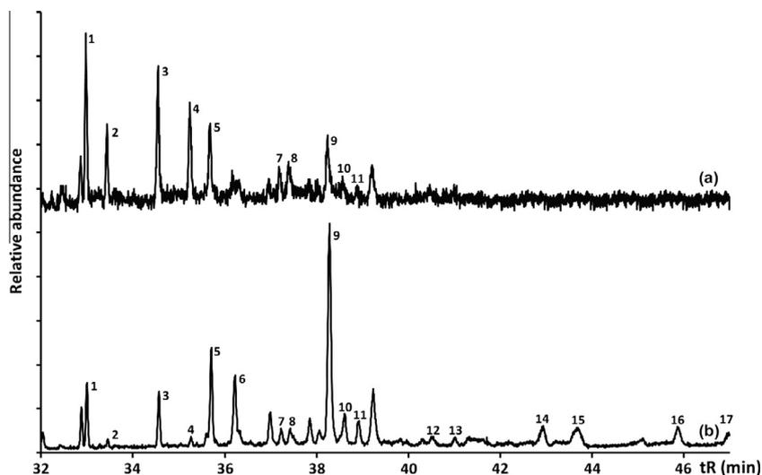
**Fig. 3.** Typical hopanoid distributions corresponding to the analysed chert samples in *Cucho* and determined  $m/z = 191$ . Refer to Table 2 for peak assignments. (a) Massive brechoid and (b) laminar.
