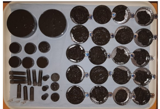
Figure A4: Sampling of the Porriño granite-doped block. Five sub-samples were taken from all four corners and centre of the formwork as it was being infilled with the mixture (two mixtures A and B poured in a total of four successive phases), for a total of 20 dose rate control samples. The sub-sampling intervals were at 12 cm from the bottom of the formwork; 22 cm of infilling (corresponding to the base of the horizontal PVC tube inserted to maintain a 8.5 cm-diameter \times 28 cm-long cavity at the centre of the doped cube); 32 cm of infilling; and at 50 cm of infilling, just 10 cm below the top of the cube.
