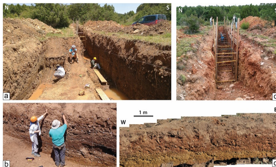
Fig. 11. Field aspect of trenches. (a) Overall view of LAG1, showing the long, southern wall (right) and the short, northern one (left). (b) Sector of LAG1 (southern wall) surveyed in detail. (c) Overall view of LAG2. (d) Photomosaic of the northern wall of LAG2 showing a massive alluvial deposit, in which no stratigraphic marker was identified.
